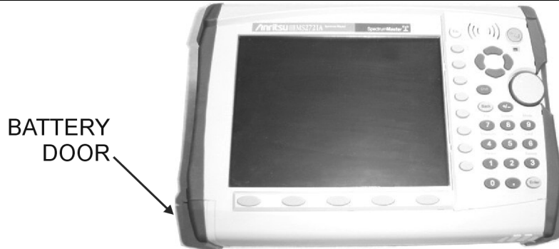
Figure 4. Battery Access Door Location
